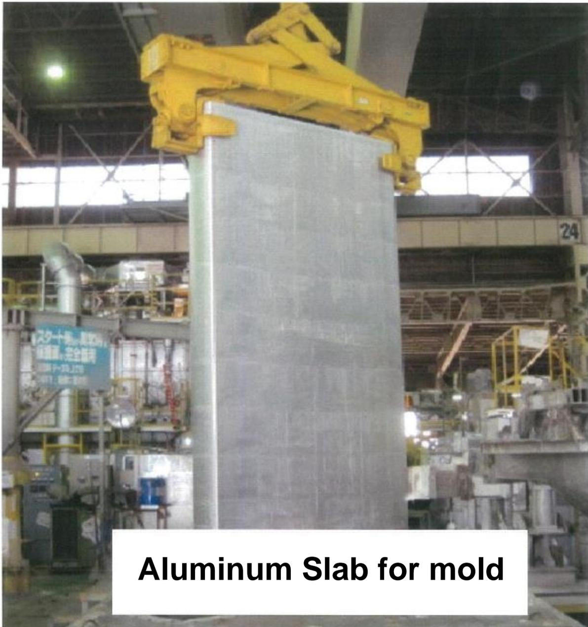
**Aluminum Slab for mold**
